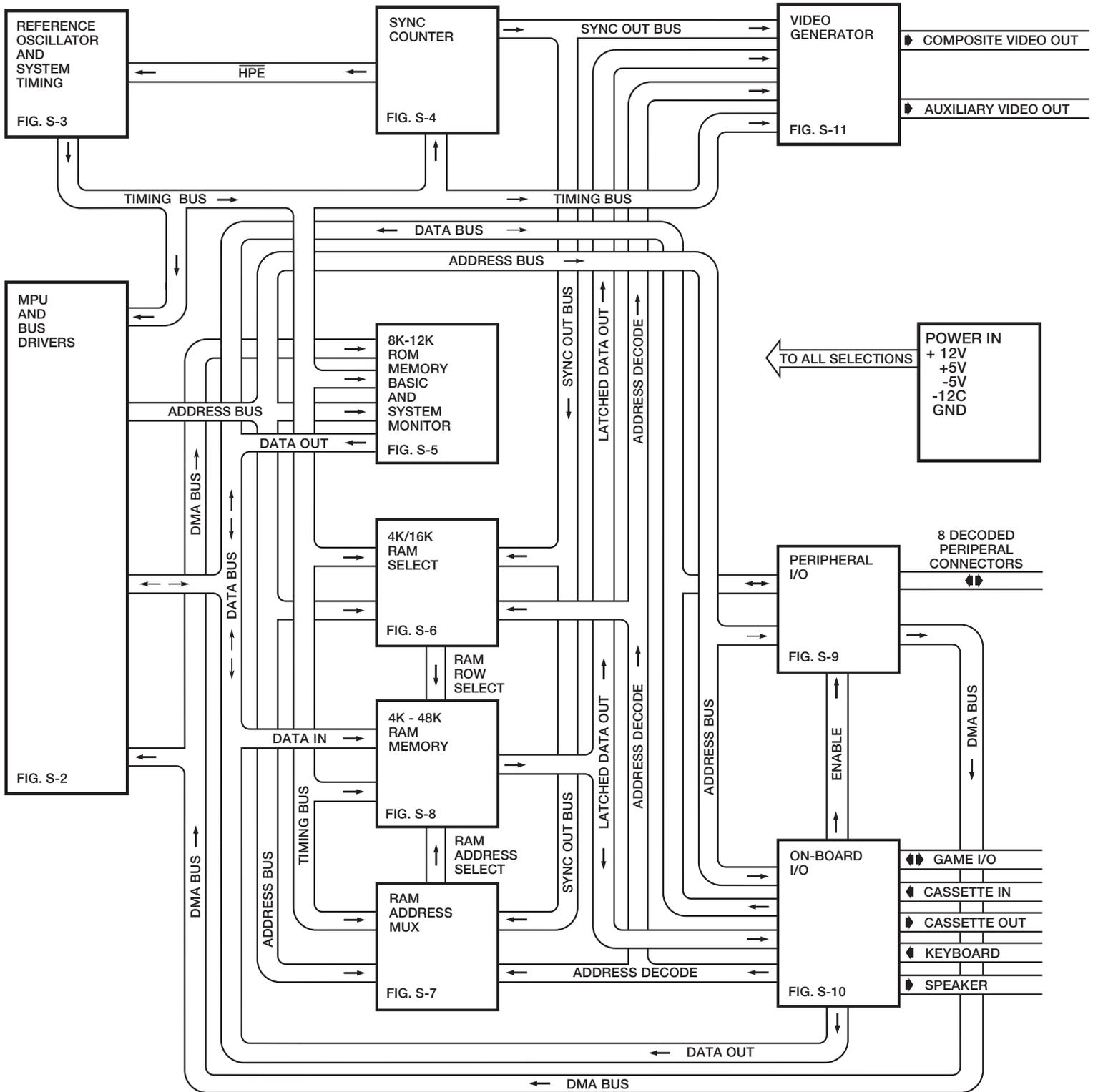
FIGURE S-1 APPLE II SYSTEM DIAGRAM
